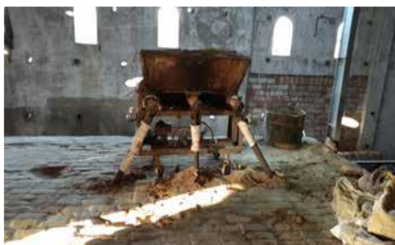
FIGURE 35 LOCALLY MANUFACTURED TRICKLE FUEL FEEDING SYSTEM USED IN MADHYA PRADESH
