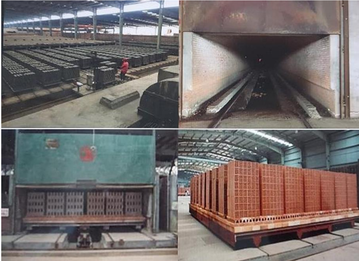
FIGURE 45 TUNNEL KILN AND DRYER
