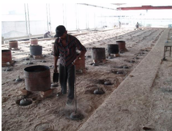
FIGURE 34 FUEL FEEDING AT ZIG ZAG KILN
