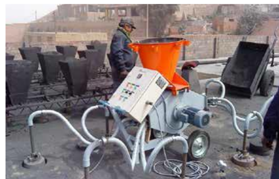
FIGURE 36 PNEUMATIC FUEL-FEEDING SYSTEM OF A EUROPEAN COMPANY 'BERALMAR'
