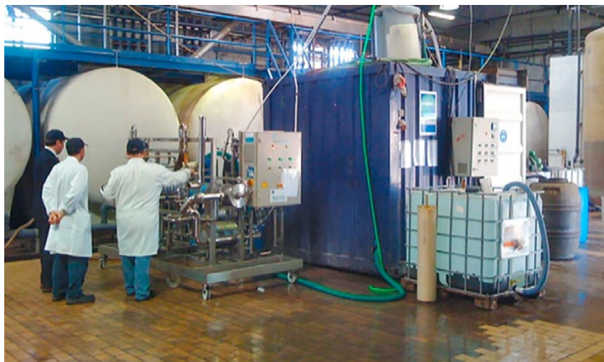
Figure 1: Mobile AQUATECTOR® Microfloat® unit for seasonal treatment of wastewater from olive processing in the context of pilot projects in Lebanon, Syria and Jordan
